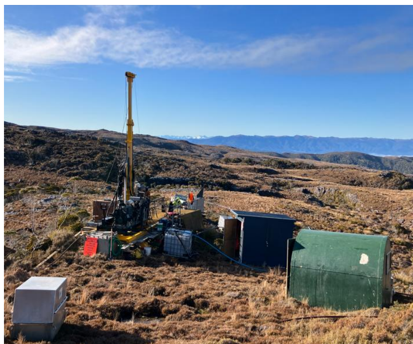
Figure 13: Helicopter supported Diamond Drilling at Mount Frederick South
