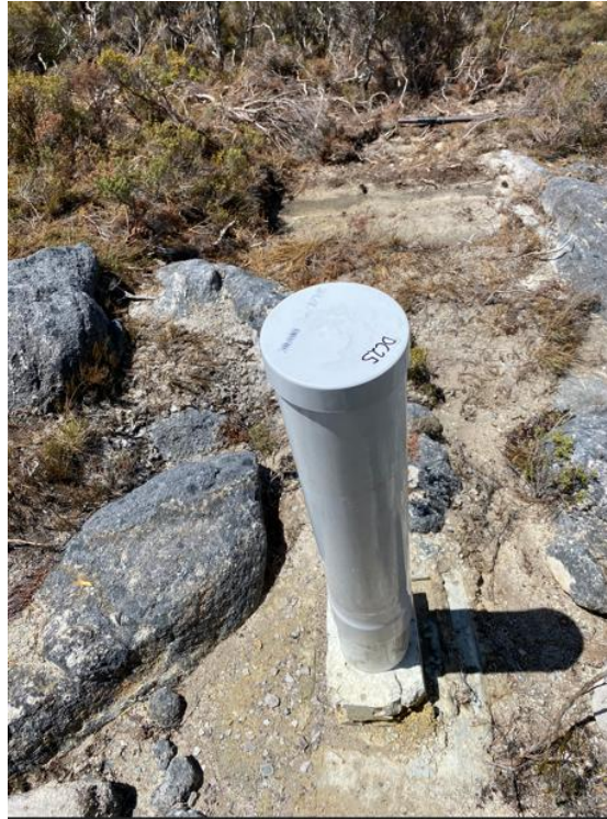
Figure 14: Standpipe installed at Mount Frederick South
