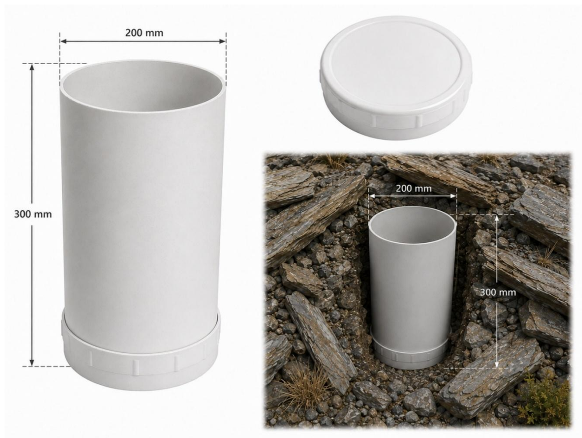
Figure 5.3. PVC pitfall trap, designed to provide a more robust, long-lasting, and lizard escape-proof trap for monitoring constructed rock stacks.
