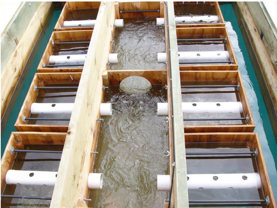
Figure 9: The FLUPSY (Floating Upweller System)
