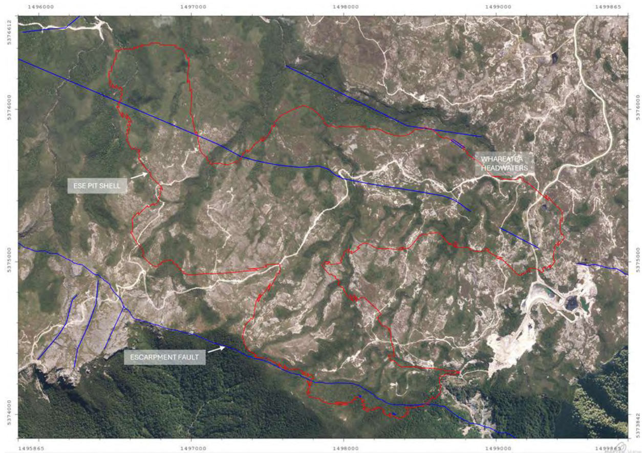
Figure 6. Aerial image of the ESE area depicting the known faults in blue , note the Escarpment fault trace in foreground.
