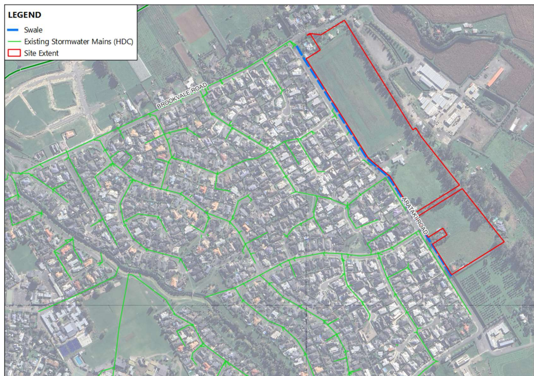
Figure 4: Existing stormwater network (Source: HDC online maps)
