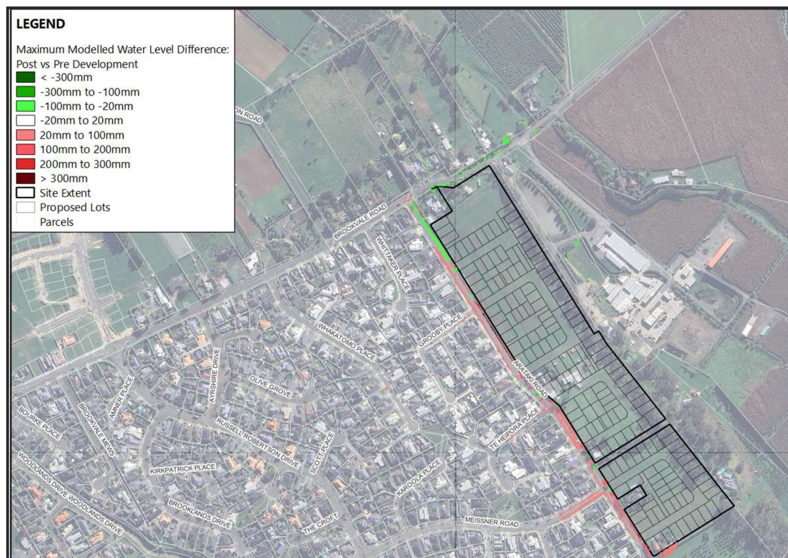
Figure 6: Water level difference (pre vs post)
