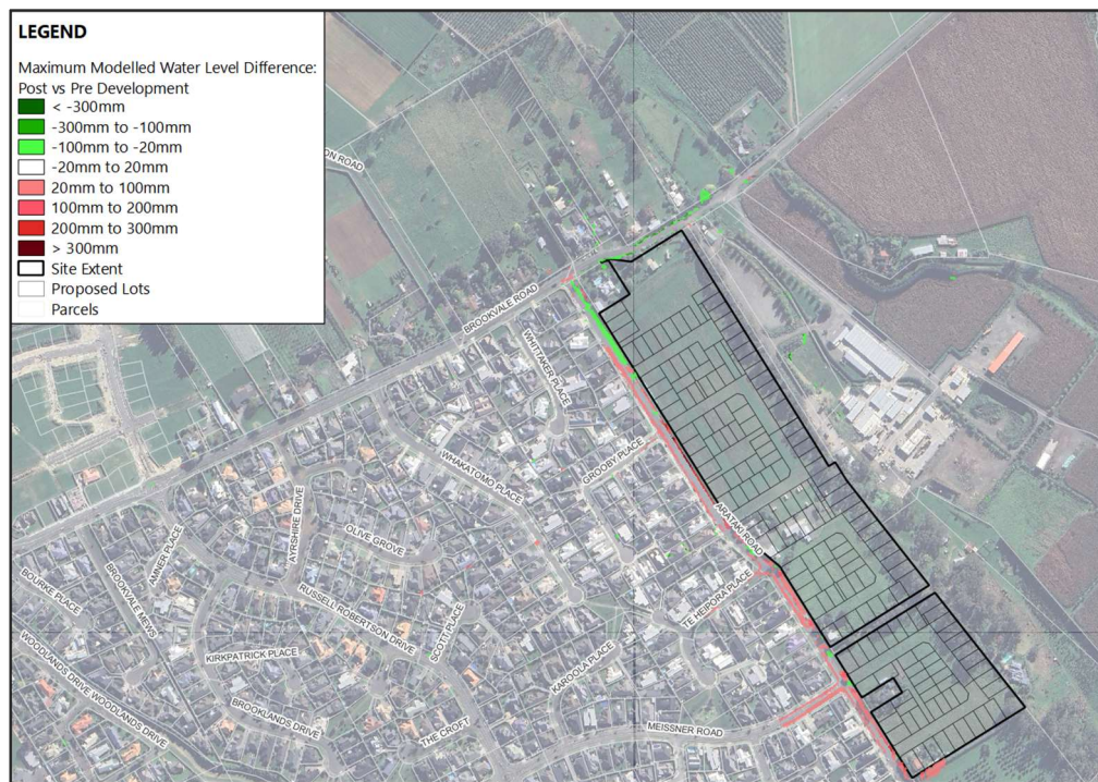
Figure 16: Water level difference plot - 100-year + RCP 6.0
