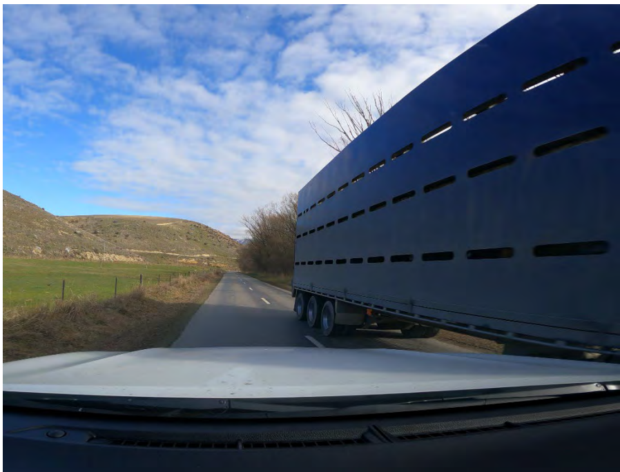
Figure 6-3: Trailer Wheels on Sealed Surface Whilst Passing
