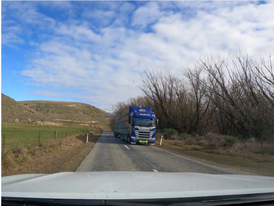
Figure 6-2: Approaching Truck Shying Away from Typical Central Tracking
