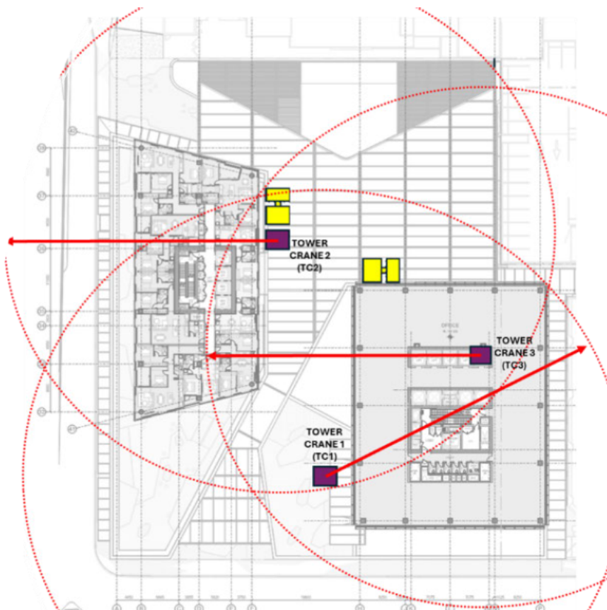
Figure 24: Indicative Crane and Hoist Locations:
