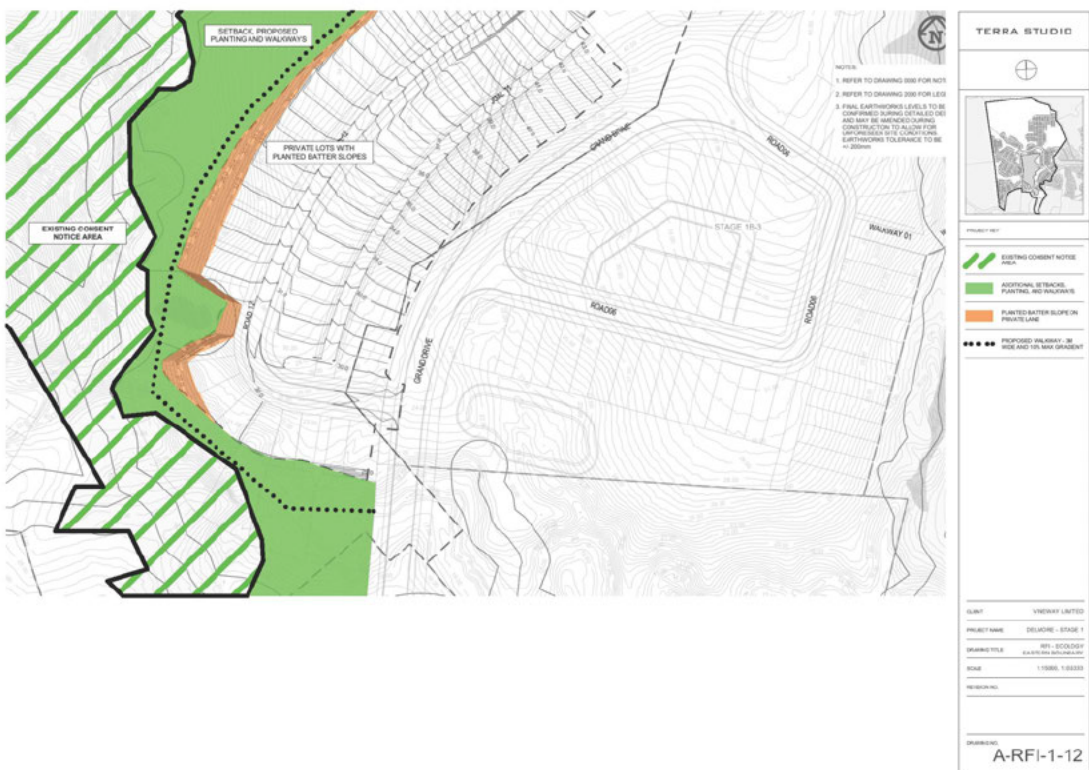
Figures 3 and 4 - Draft earthworks drawings by Mckenzie & Co showing proposed planting, walkways and batter slopes.
