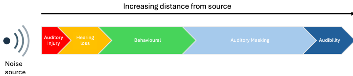
Figure 3: Effects categories in order of increasing distance from the noise source.
