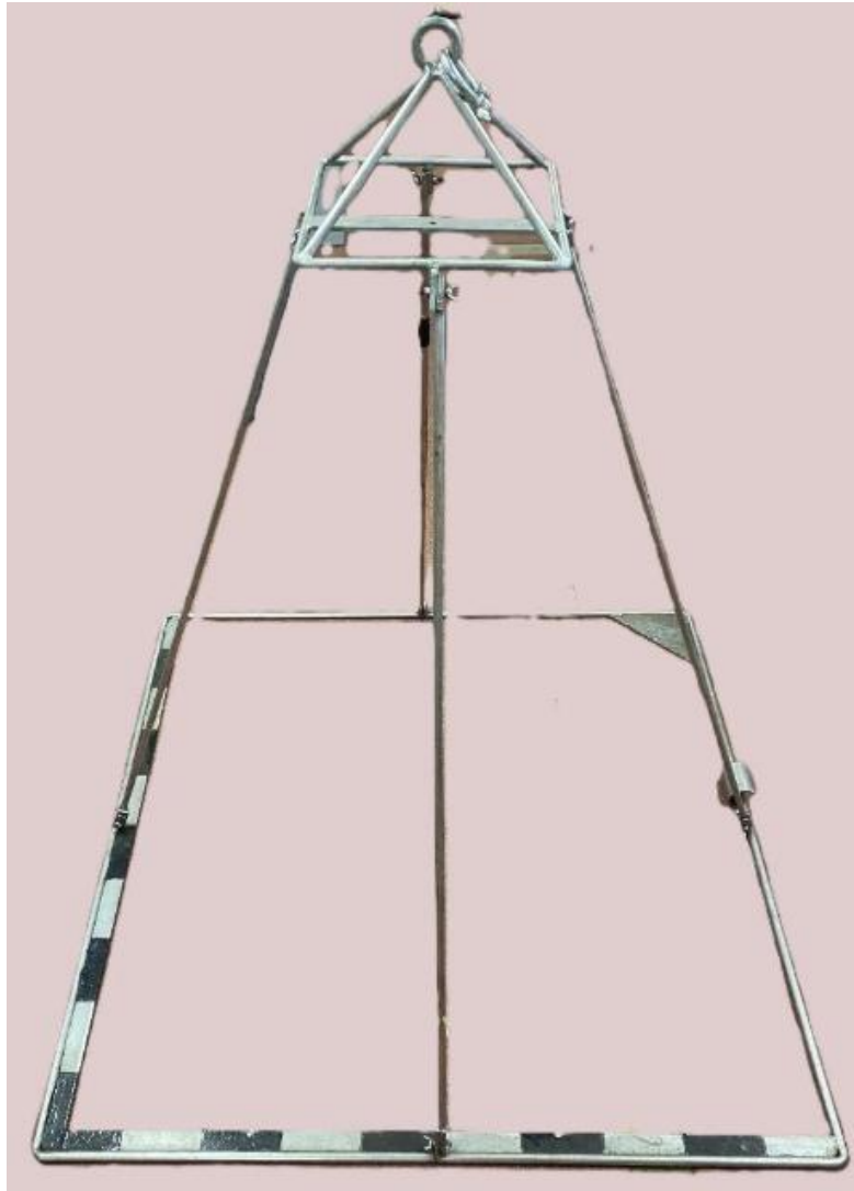
Figure 4-10: MBL's drop camera frame. Image credit: Shayne Elstob, MBL.
