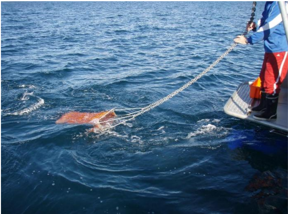
Figure 4-12: Epibenthic dredge being deployed. Image credit: Simon West, Bioresearches.
