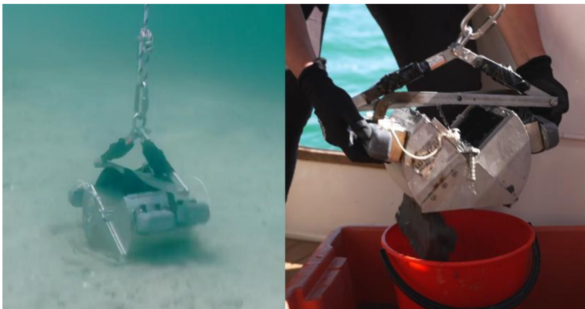
Figure 4-11: Modified standard ponar grab. Left: collecting a sediment sample on the seabed. Right: Sediment sample being emptied into a bucket. Image credit Simon West, Bioresearches.
