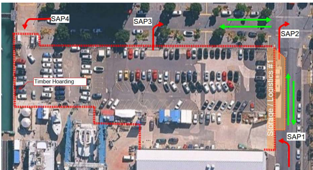
Figure 7: Site Layout for Construction Phases
