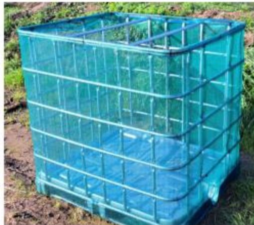
Example of a 'box' type fish screen.
