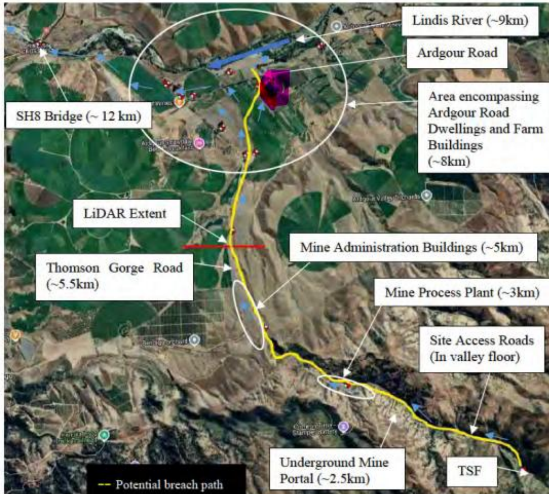
Figure 1: Potential breach flood path, items of interest and approximate distance downstream (Source: Google)
