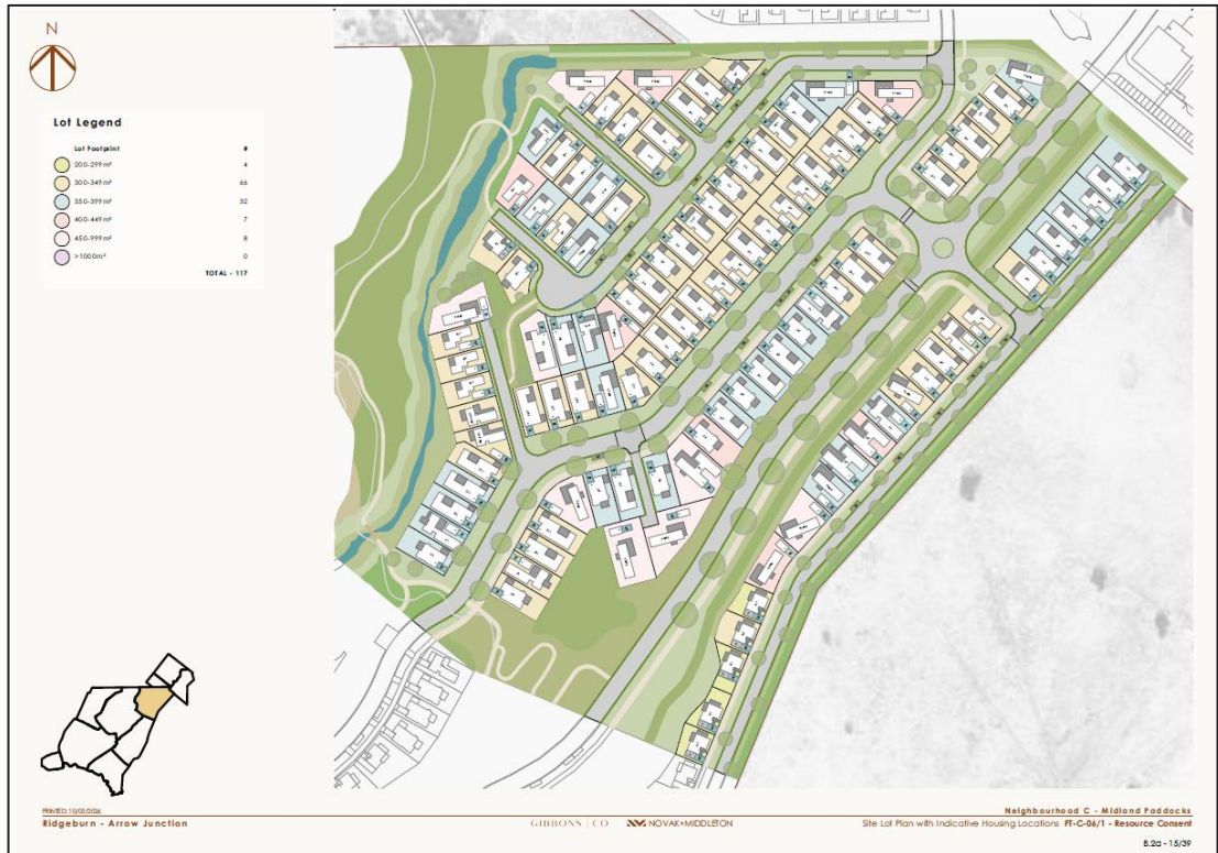
Figure 16: Midland Paddocks Neighbourhood (Indicative dwelling layout). Source: Ridgeburn Residential Neighbourhoods B C D E Plans - Family Housing (Refer Appendix 7)
