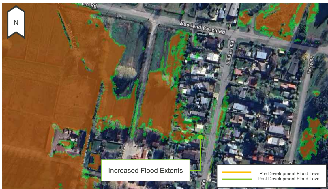
Figure 2-33 Woodend Beach and Stalkers Road Flood Levels
