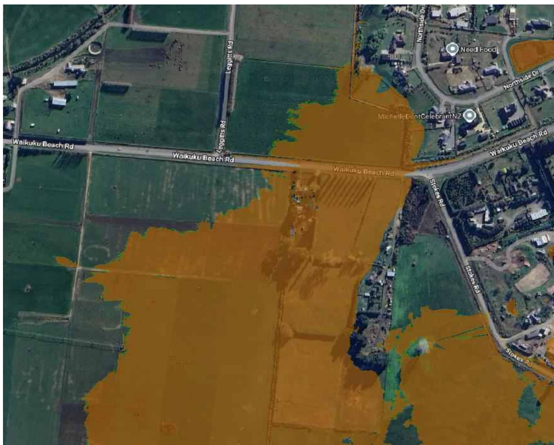
Figure 2-26 Flood Extents results from the Volumetric Assessment (Brown– Pre-development Scenario; Green – Mitigation Scenario)
