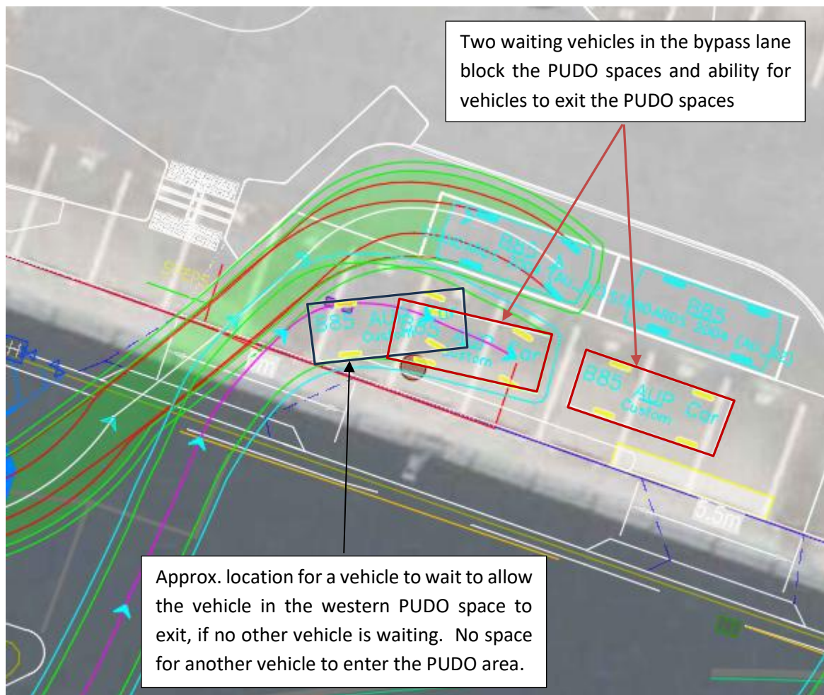
Figure 1 - Vehicles waiting in PUDO bypass lane
