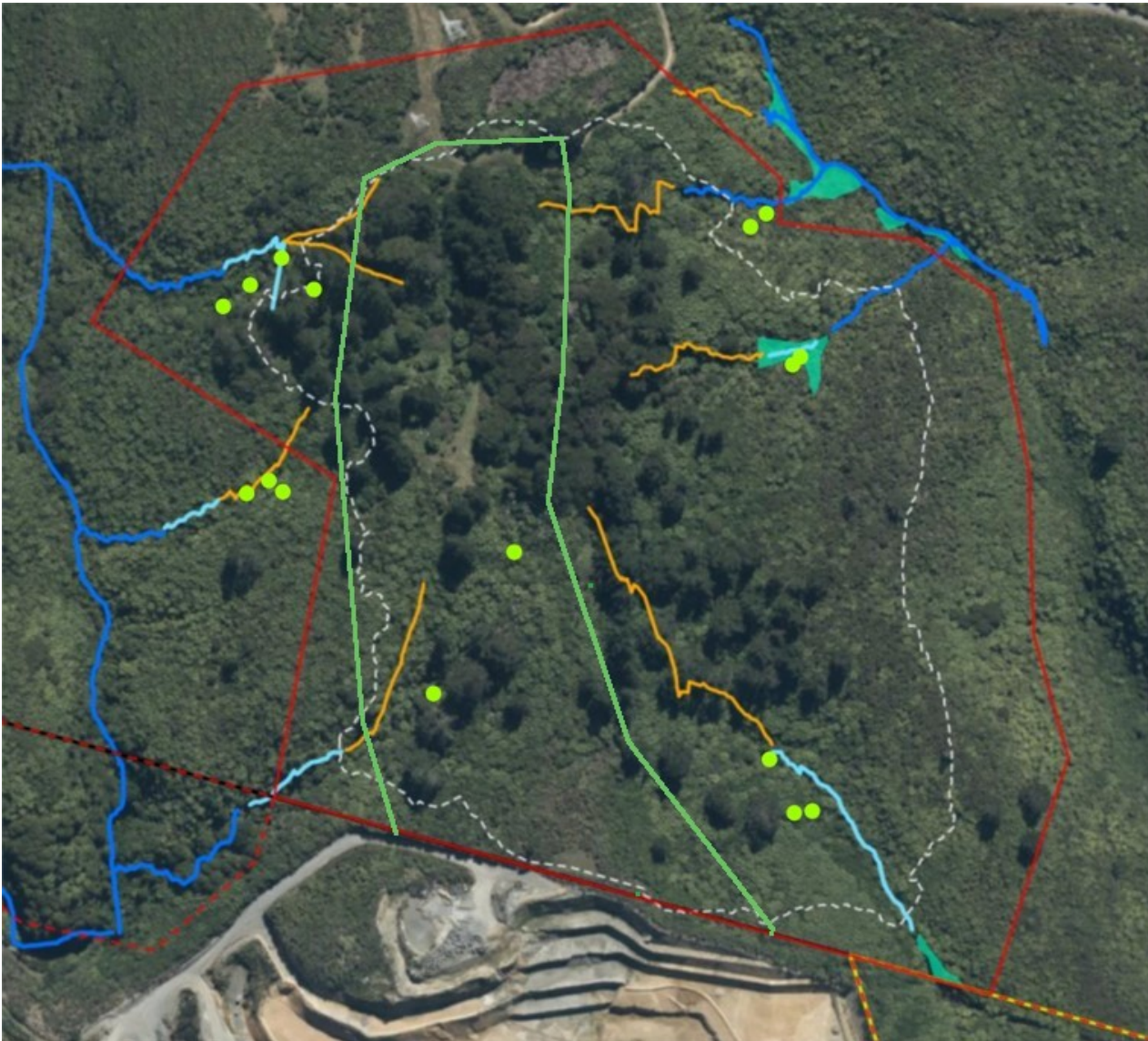
Figure 4: Based on Fig 2.1 from the Hydrology Report (Appendix B9), showing stream courses in blue/yellow, and the proposed land exchange area in red. We have added green dots to show swamp mair locations, and a green line indicating a reduced OBDA which would preserve threatened flora, wetland and lizard habitat, and preserve public recreation access to most of the area.
