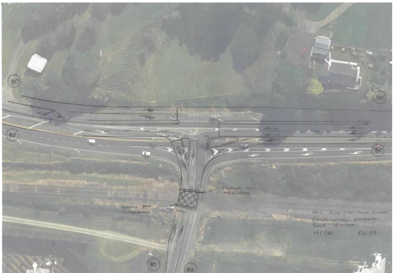
Figure 5-15: Proposed design signalised intersection (source: Boffa Miskell)
