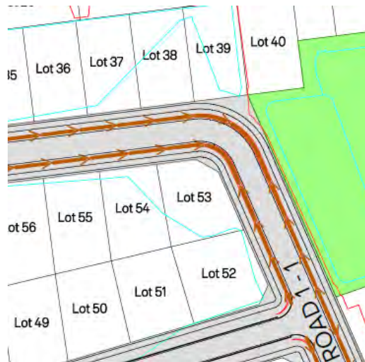
Figure 30: Lot 53 Non-Compliant Sight Distance
