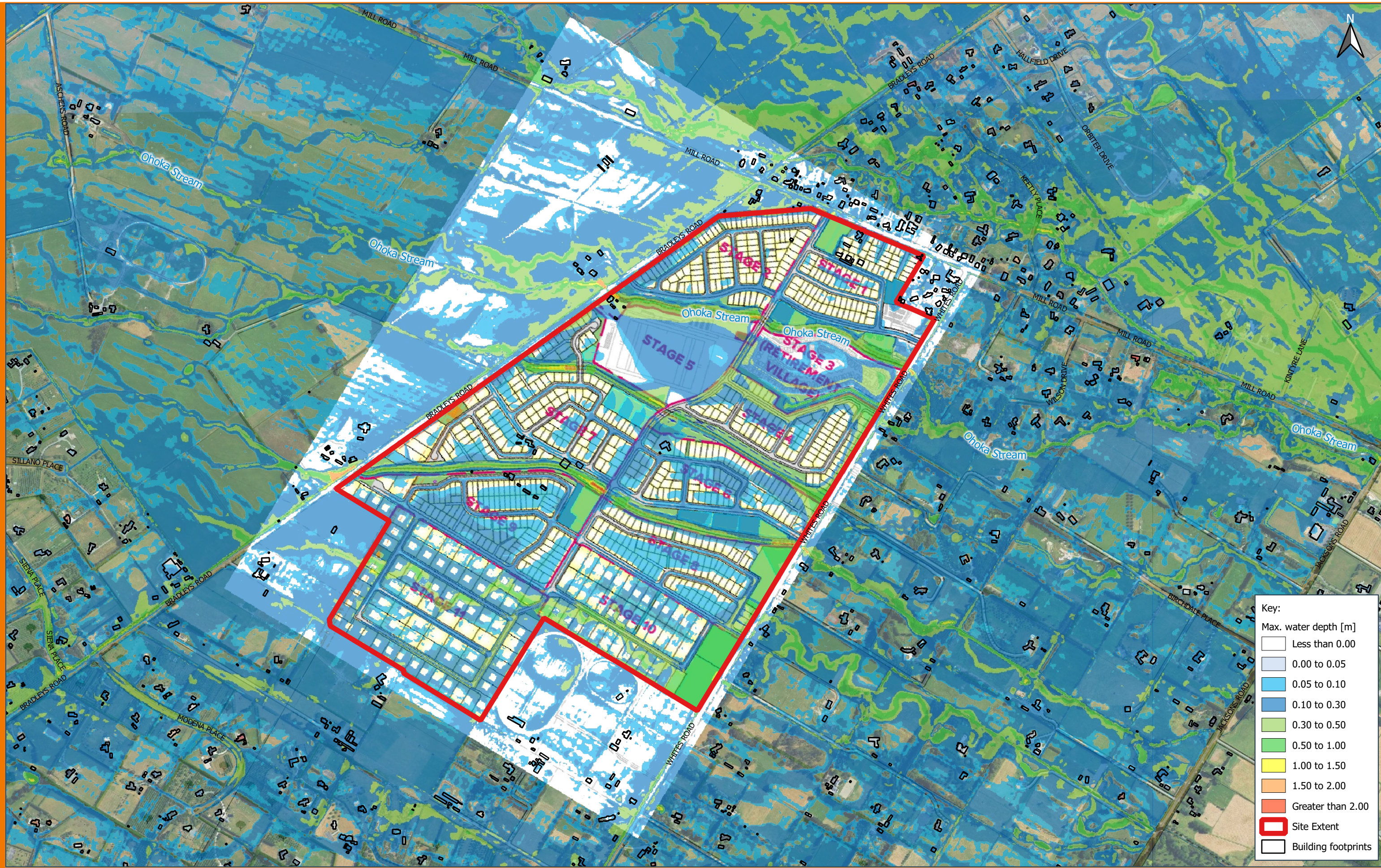
pdp Figure A5, Post-development flood depths for the 200-year event with climate change (D02_200YR_Post). Depths less than 50 mm not shown
