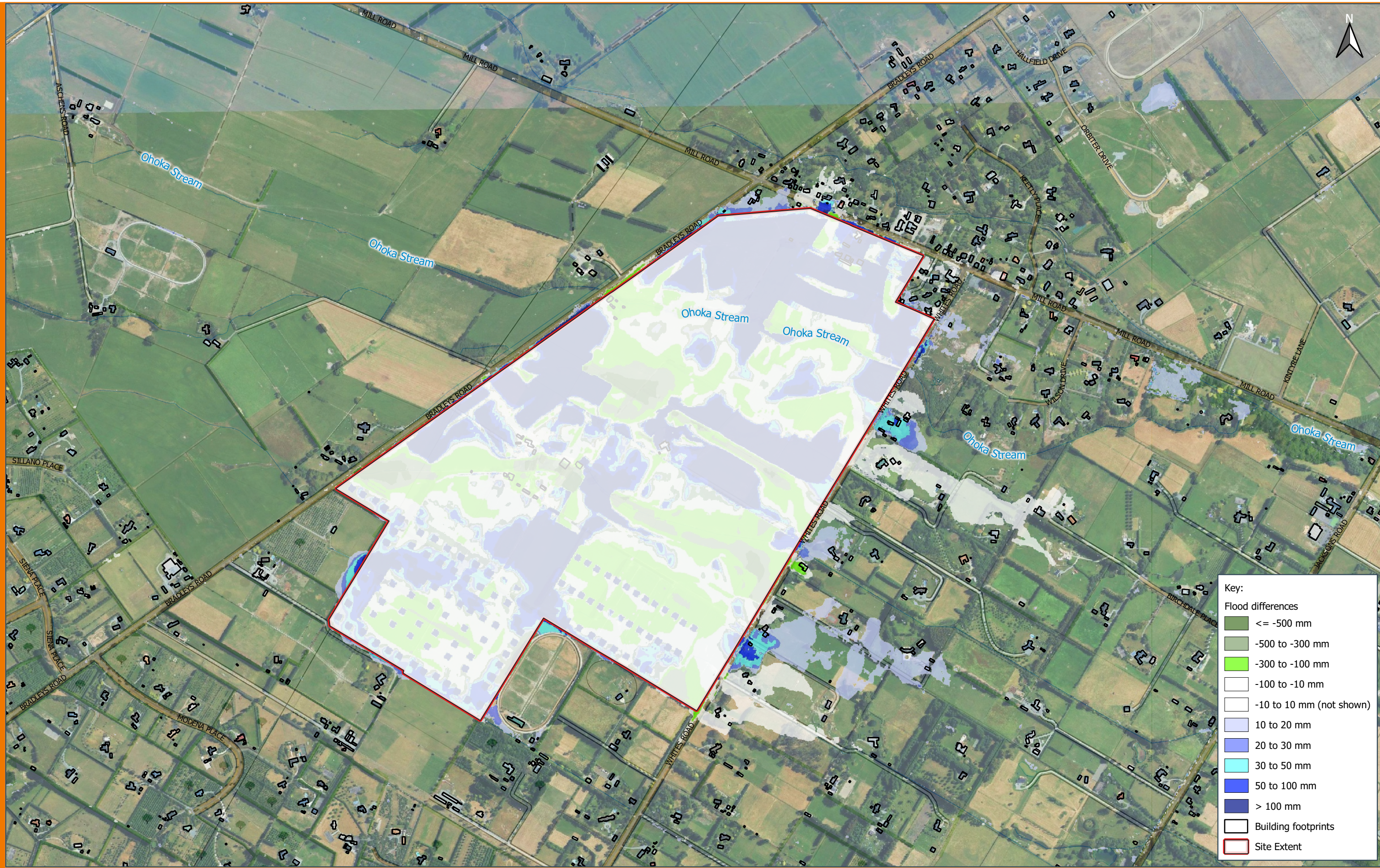
pdp Figure A6, Flood difference (post-pre development) for the 200YR event with climate change. Differences less than 10 mm are not shown
