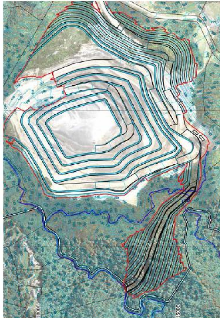
Figure 6: Proposed stream diversion design (indicative)
