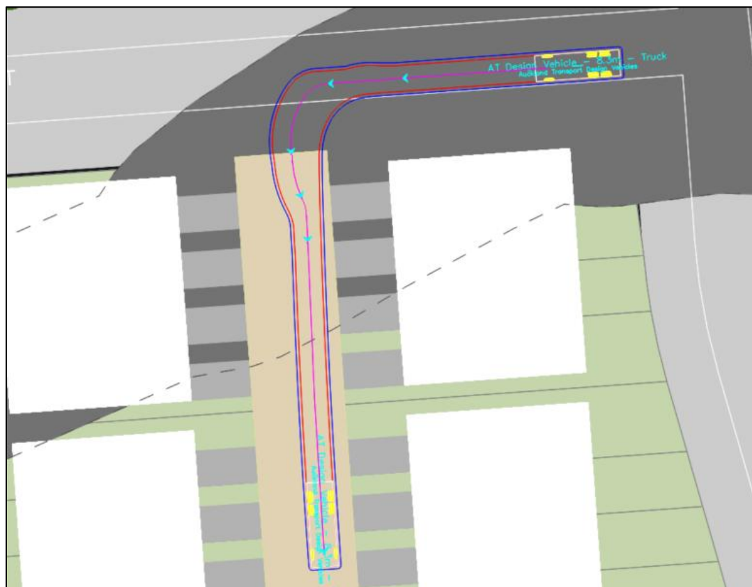
Figure 7-61: Super lot E3 - loading space tracking (inbound)
