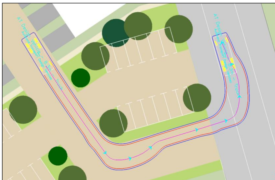
Figure 7-62: Super lot E3 - loading space tracking (outbound)
