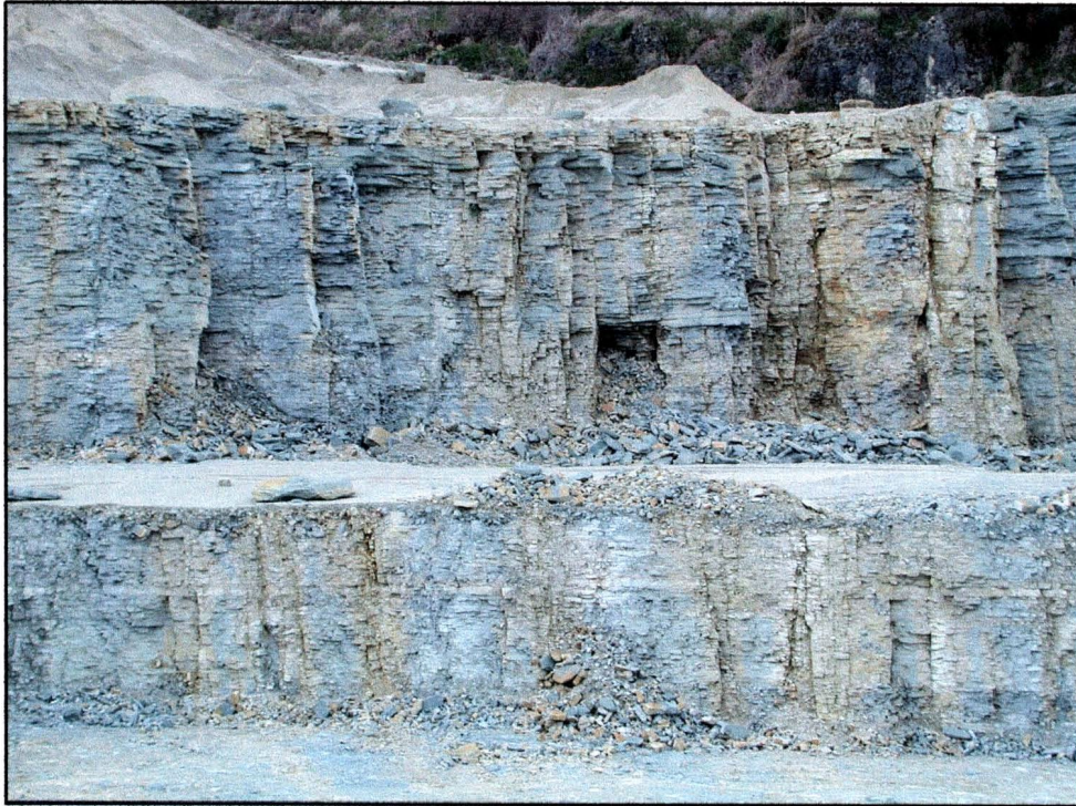
Figure A5: Fractured limestone on quarry wall (Frostad, 2004)
