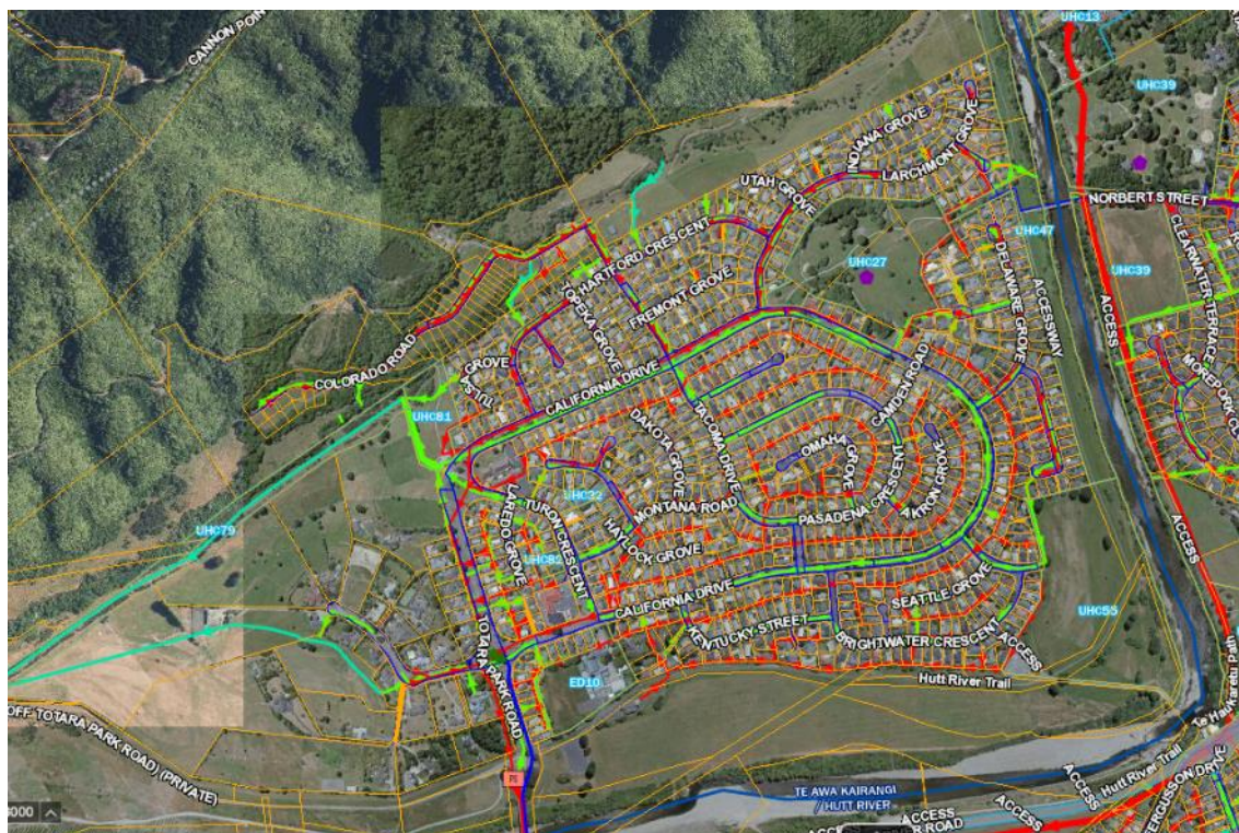
Figure 5. UHCC piped water system map showing that the stream and two drainage areas of the pasture are taken into the below ground piping and fish passage would need to exit the Hutt river come up the council drainage system enter the pipes and access through good navigation the stream (a journey of over 400m).
