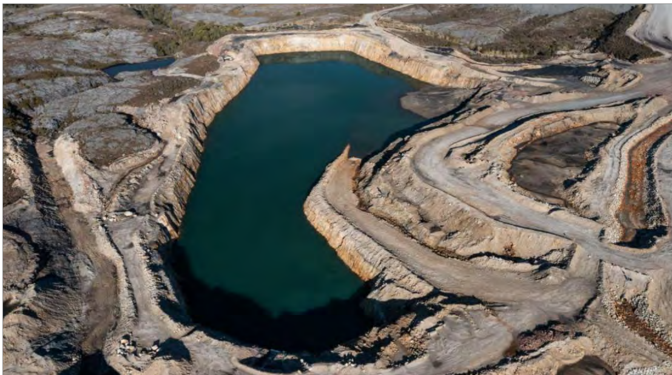
Figure 3-12 McCabes AMD treatment sump - operational since 2024 (source: Bathurst 2025b)
