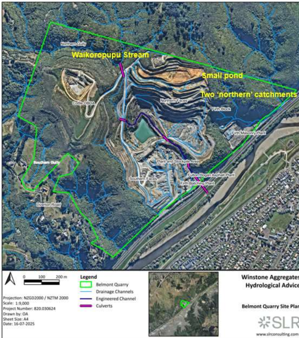
Figure 2.2: Belmont Quarry drainage and imagery.
