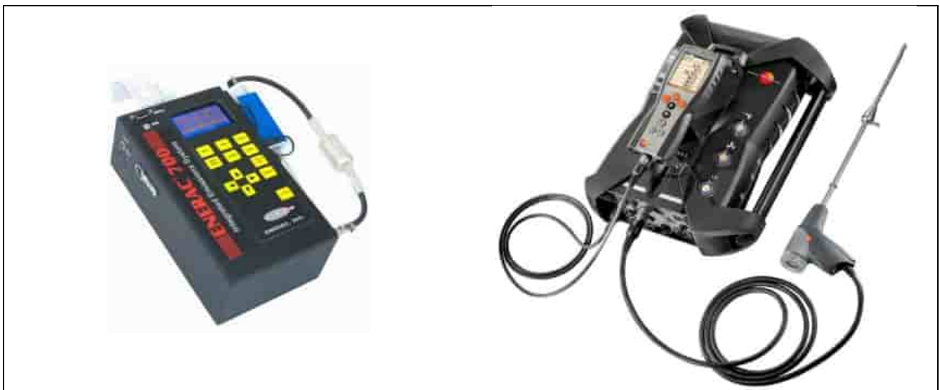
Figure 5 Combustion Gas Analysers
