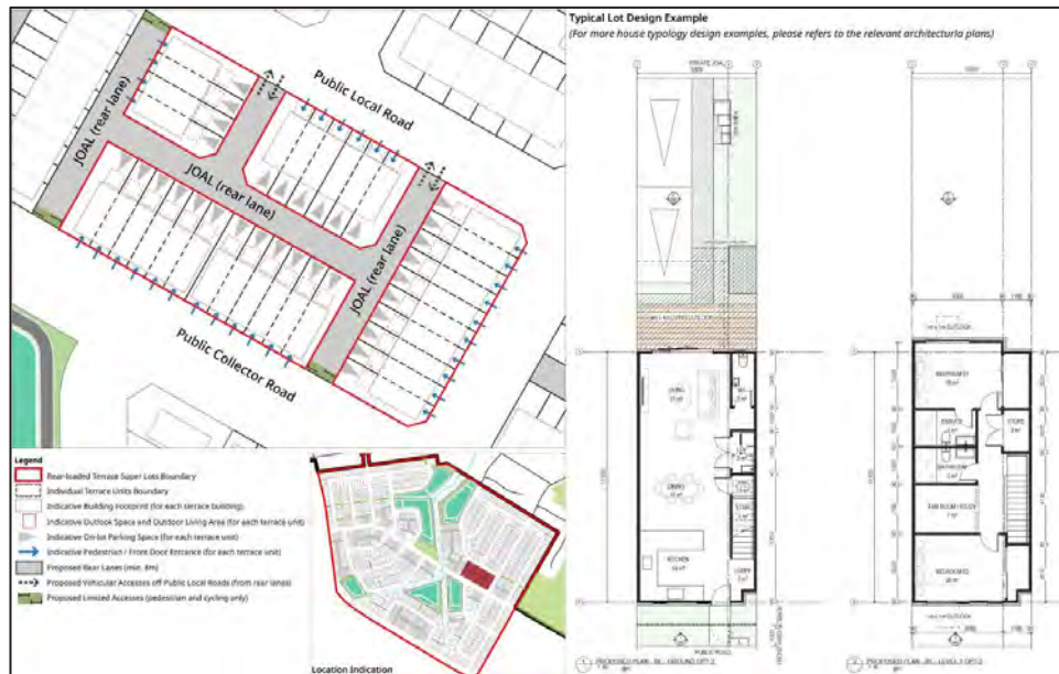
Figure 14 Typical Rear-loaded Terrace Dwellings Development
