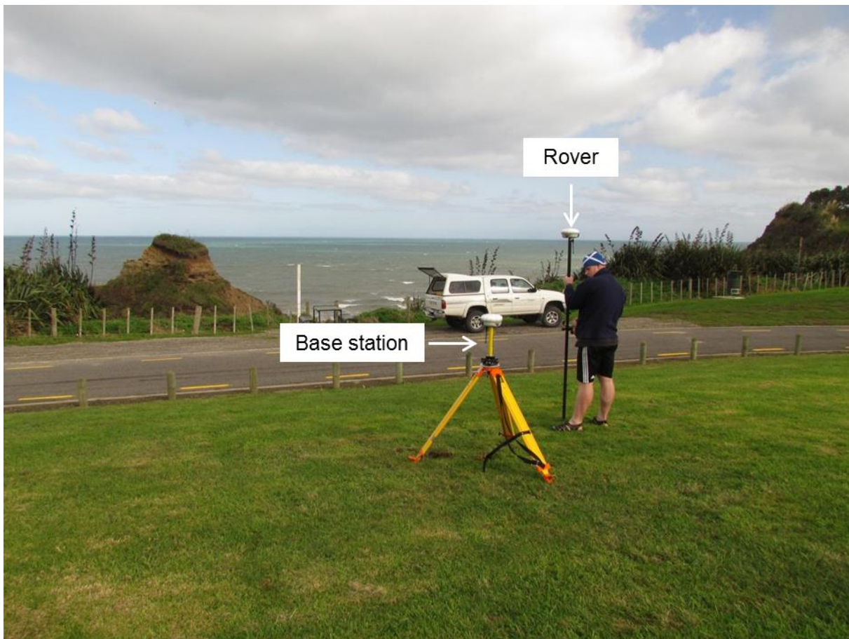
Figure 2-1: Photo showing RTK GPS base station and rover setup at Hawera.
