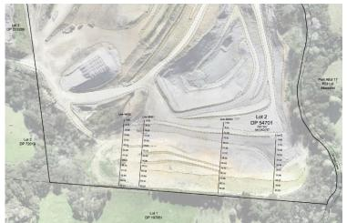
of three rotary cored machine boreholes to depth of up to 27.5m, in the alignments depicted on the inset (left). These tests are located east of the proposed 'Yard Base' (blue area).
