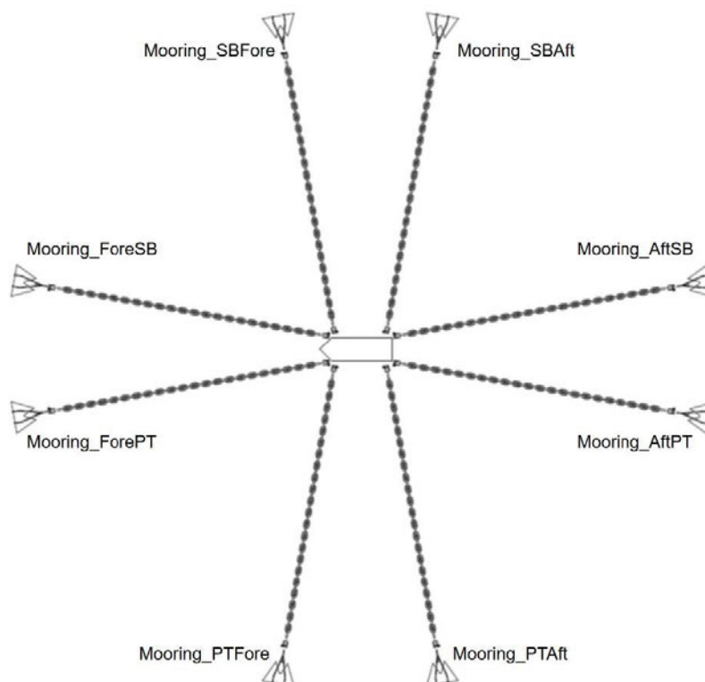
Figure 12: Mooring layout for feed barge (not to scale).
