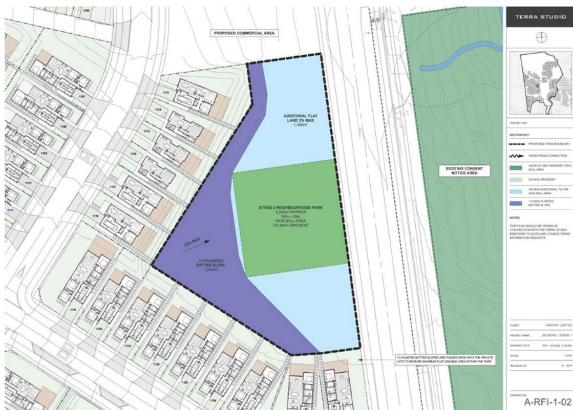
Figure 3 – Stage 2 park amended slightly since the initial application to suit the new collector road width and roundabout.
