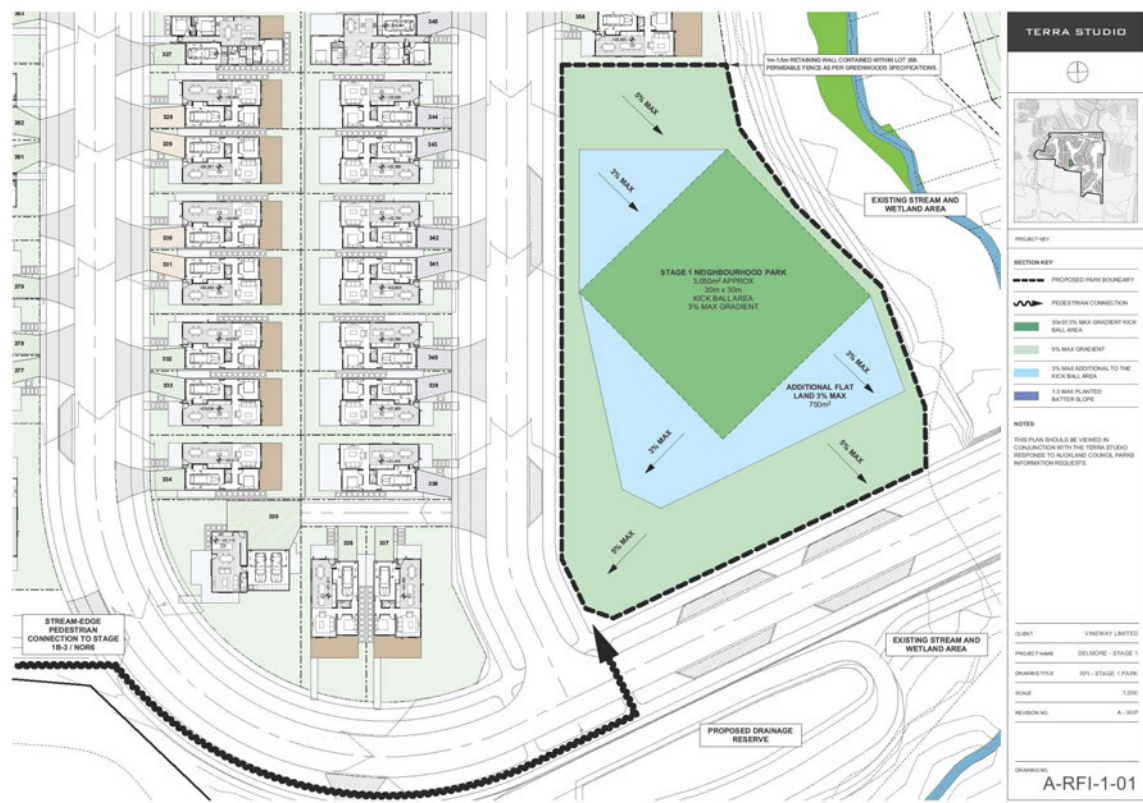
Figure 1 - Stage 1 park with an additional 750m2 of 3% max. gradients outside of the 30x30 kickball area highlighted in blue
