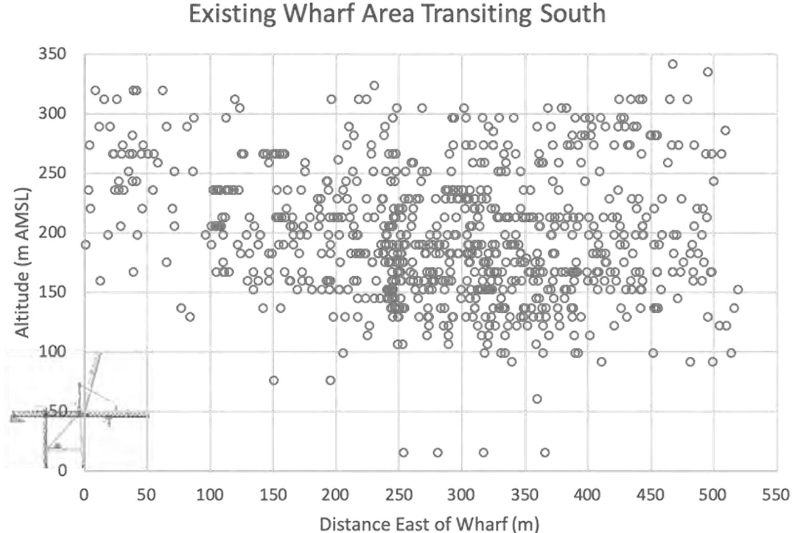
The cross section (Figure 06-10) shows that similarly a number of aircraft are flying below the height of the proposed cranes while passing the wharf, a greater proportion are flying at near to that height (at or below 150m).
