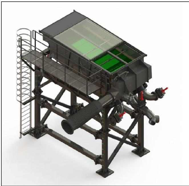
**Figure Nine: 3 D Plan of sand 'screening deck' on the William Fraser**
