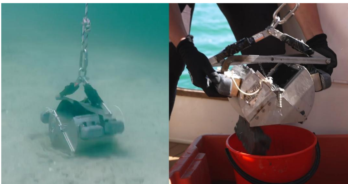
Figure 7: Modified standard ponar grab. Left: collecting a sediment sample on the seabed. Right: Sediment sample being emptied into a bucket. Source: Simon West, Bioresarches, personal communication.
