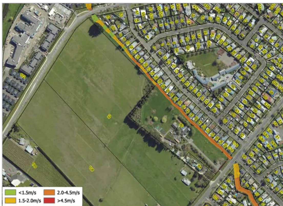
Figure 6: Velocity bands for the 2% and 1% AEP storm events (source: HDC landowner tools and guides)
