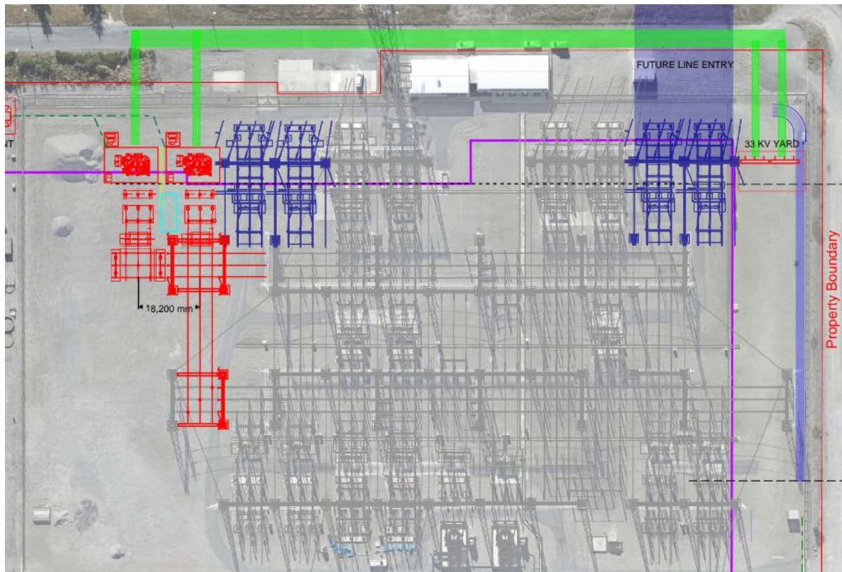
Figure 4.9: Equipment Arrangement within the Twizel Substation
