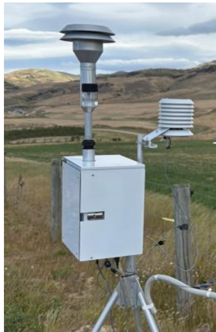
Figure 8: Photograph of real time dust monitoring equipment
