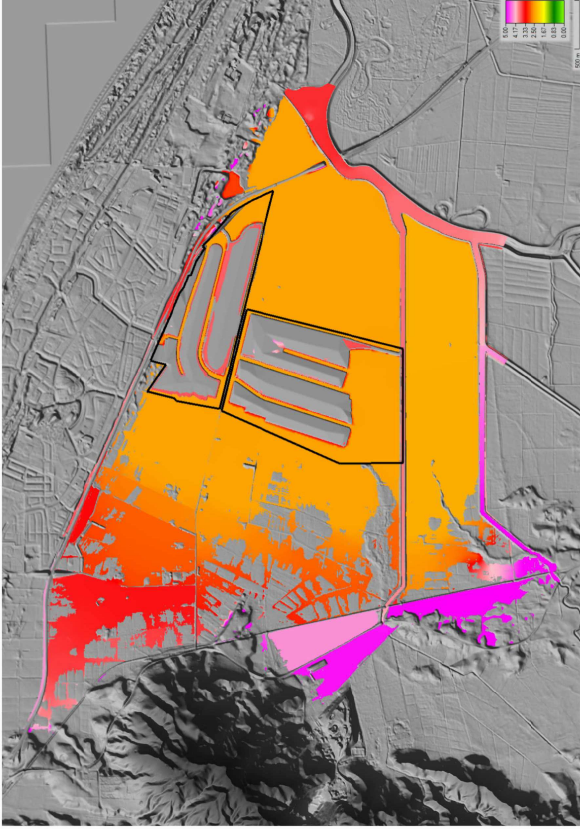
Figure 80 - 100yr ARI 3.68°C Climate Change SLR 1.59m, Post-Development Water Surface Elevation (m, NZVD16)
