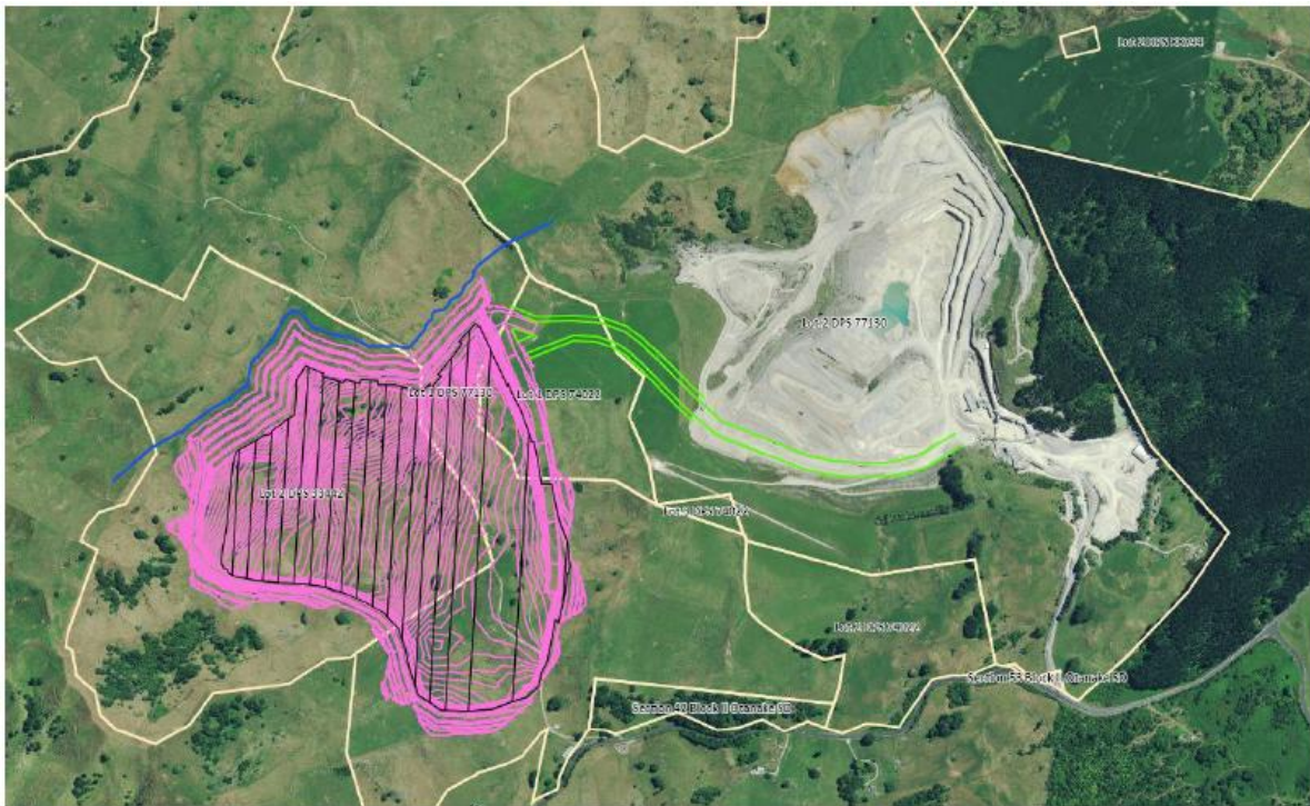
Figure 1-1: Graymont Quarry (Lot2DPS77130) and the proposed haul road (green), proposed Southern Catchment Pit extent (pink) and divide line (blue). Figure retrieved from (Instream Consulting, 2024)
