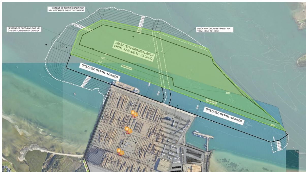
Figure 3b: Stage 2 Dredge (green) (Source: Northport).
