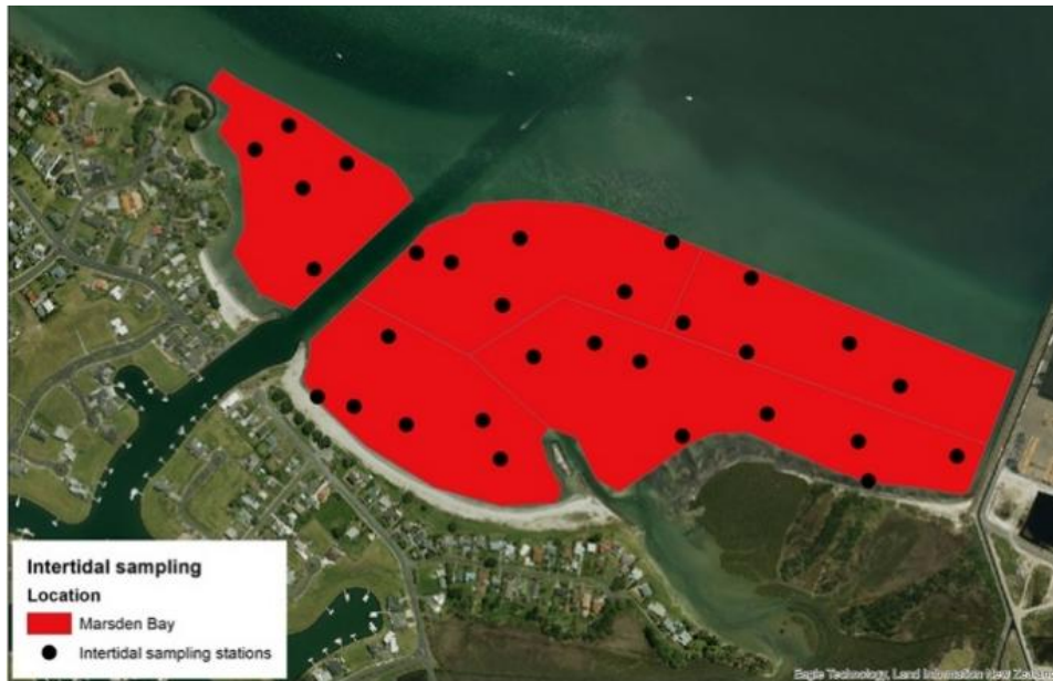
Figure 9: Indicative sample design for inter-tidal sediment and infauna monitoring.
