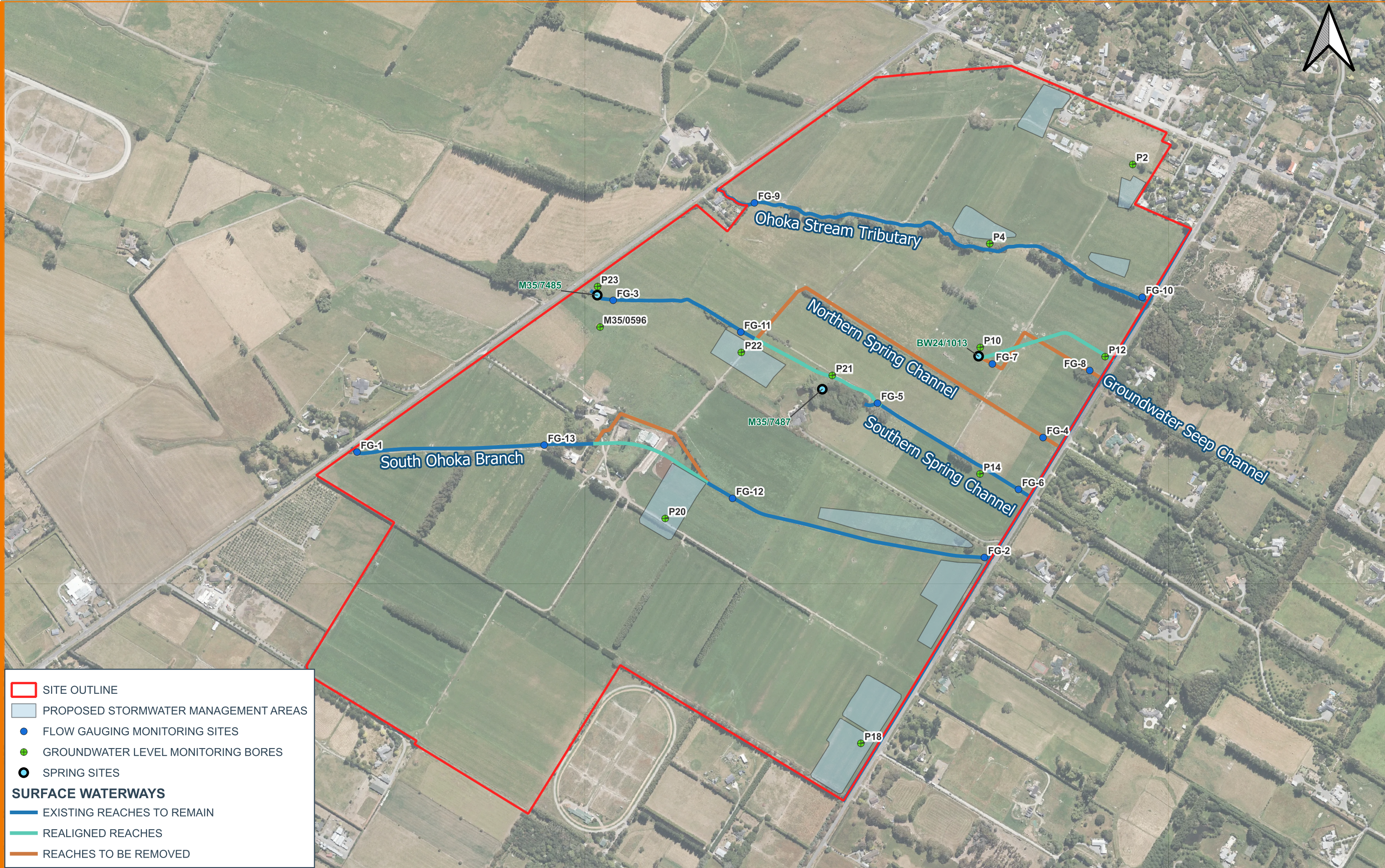
FIGURE 01: PROPOSED SURFACE WATER AND GROUNDWATER MONITORING SITES FOR CONSTRUCTION EARTHWORKS
