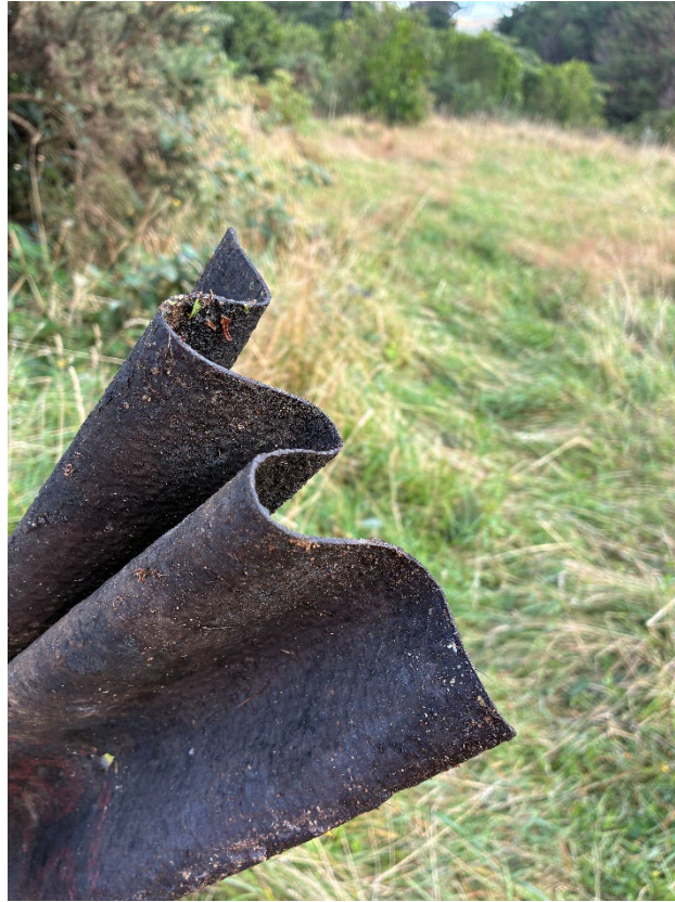
Photograph 7: Photo of potential asbestos at SS01.
