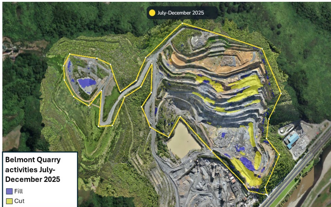
Figure 10: Location of Cut and Fill Activities at Belmont Quarry between July to December 2025
