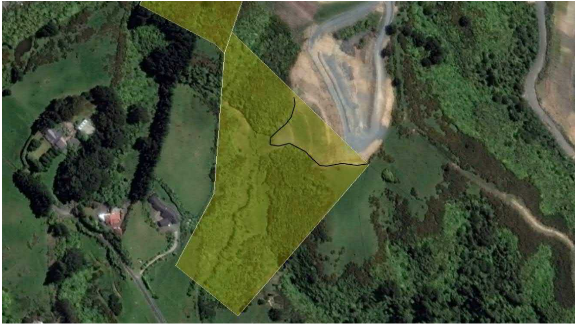
Figure 7-1: Southern Gully Parcel [yellow] illustrating extent of Cottle OBDA fill placement [black line]
