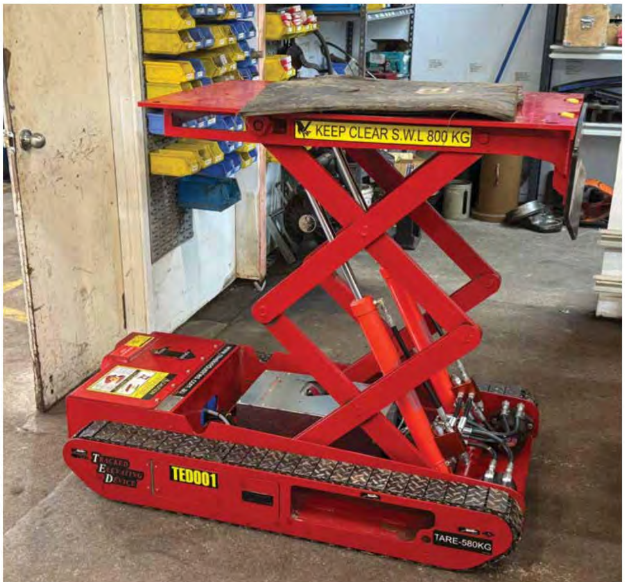
Tracked elevating device – remote-controlled, all-terrain lift for safely handling heavy mining equipment components.
