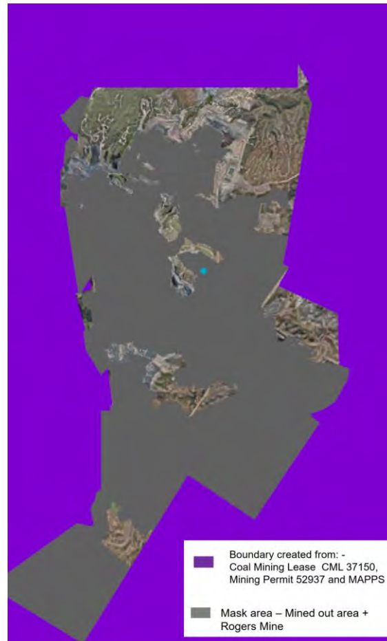
Figure 27: Surface Constraints Utilised for Stockton Pit Optimisation
