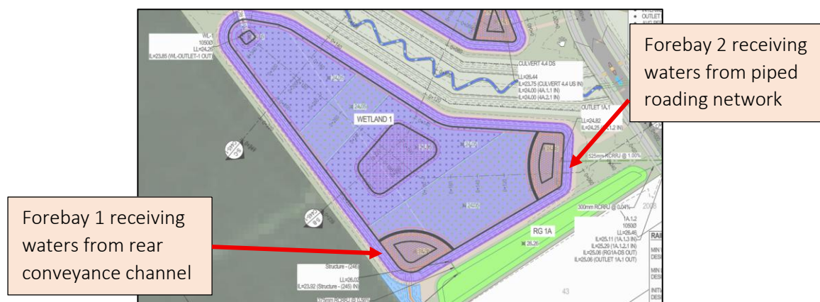
Figure 12: Typical Additional Wetland Forebay Configuration
