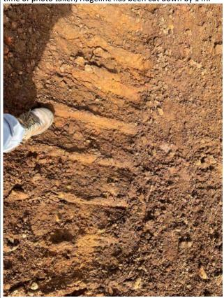
Track rolled material comprising clayey silt with basalt gravel inclusions.
