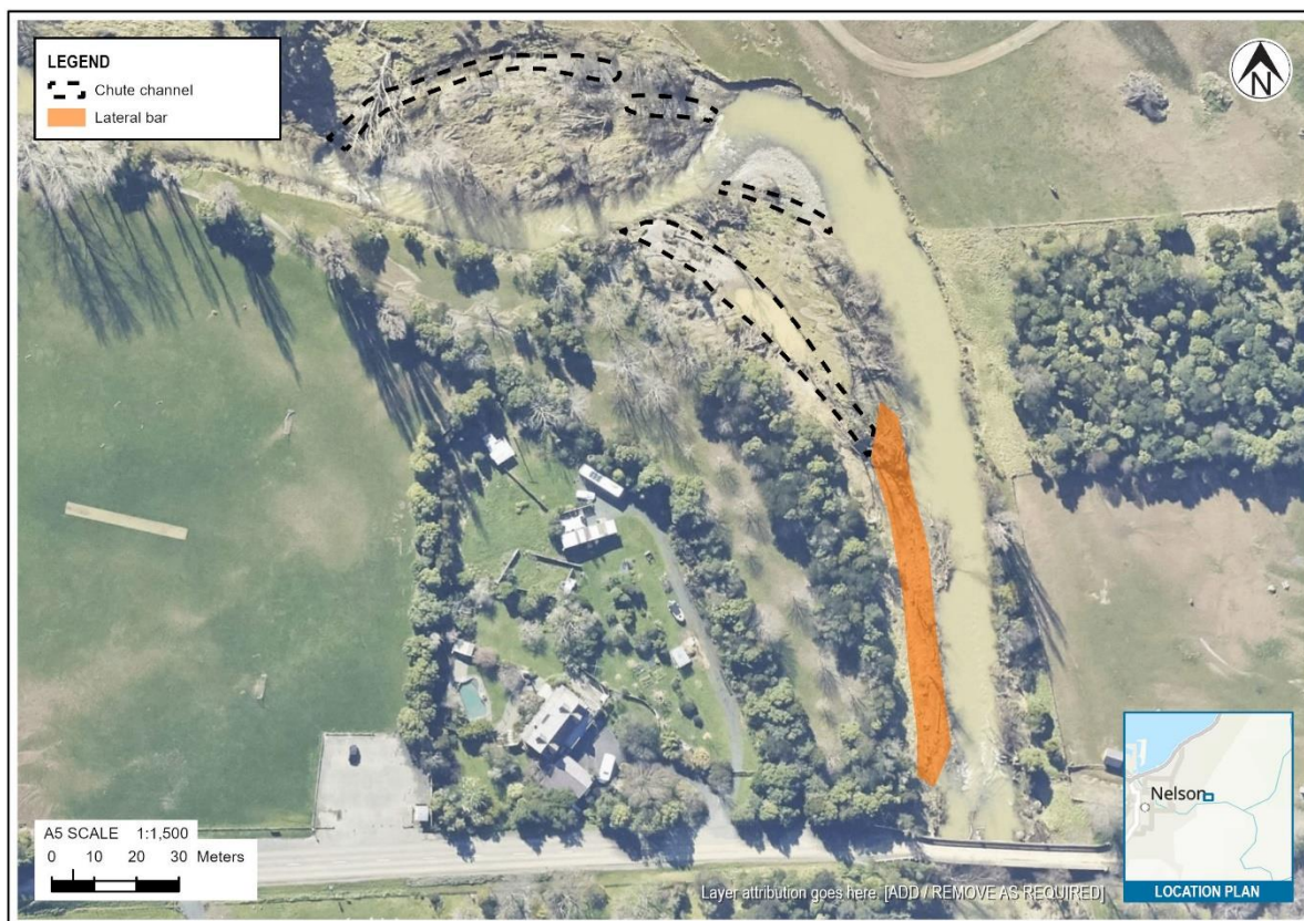
Figure 2.6: Plan of the upper Gibbs – Dennes reach, showing the lateral bar and chute channel.
