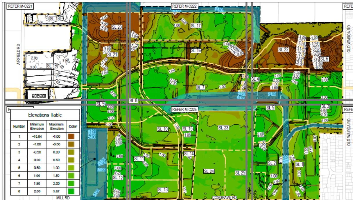
Figure 1: Cut/Fill Plan (Source: Maven, Drawing No:M-C210, Rev: A, February 2025)
